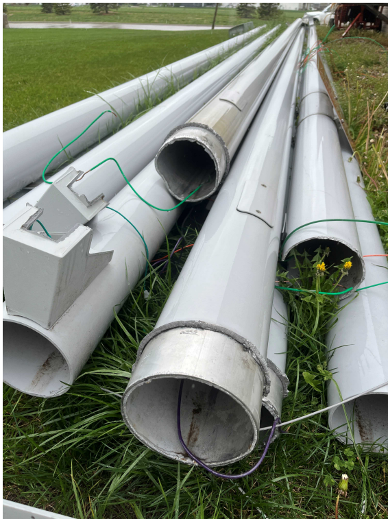
Failed light pole bases and base castings
