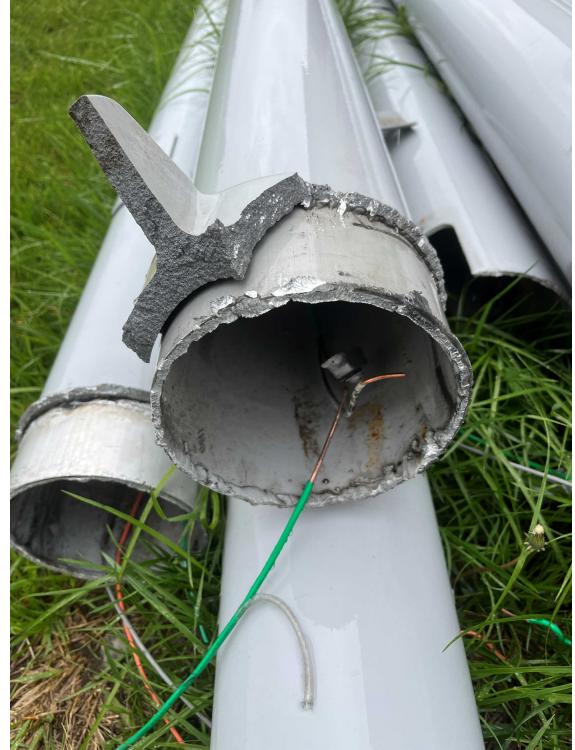
Failed light pole bases and base castings
