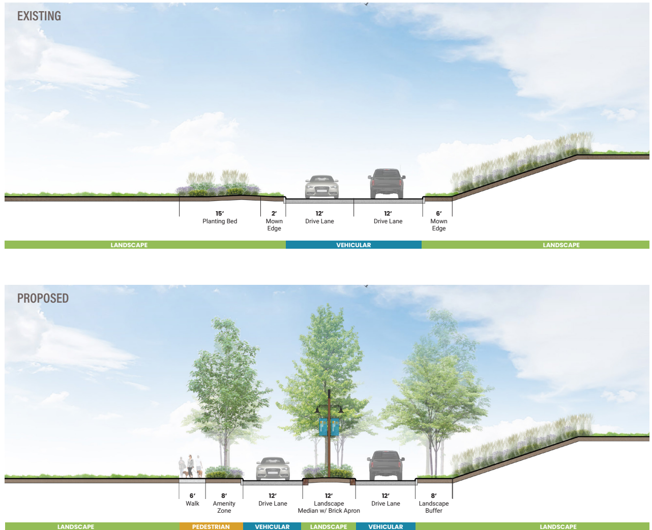
FIGURE 4.05 / SECTIONS OF EXISTING AND PROPOSED GATEWAY IMPROVEMENTS AT 1ST STREET LOOKING WEST
