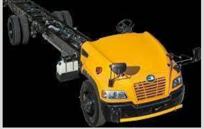
Purpose built Blue Bird OEM chassis.
