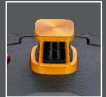
Main LiDAR The main LiDAR sensor array used in mapping and navigation
