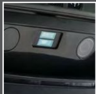
Main Camera Used to identify obstacles and people, and navigate around them
