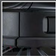
Touch Shield A buffer that, when touched, causes the immediate stop of the robot
