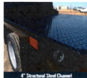
4" Structural Steel Channel
