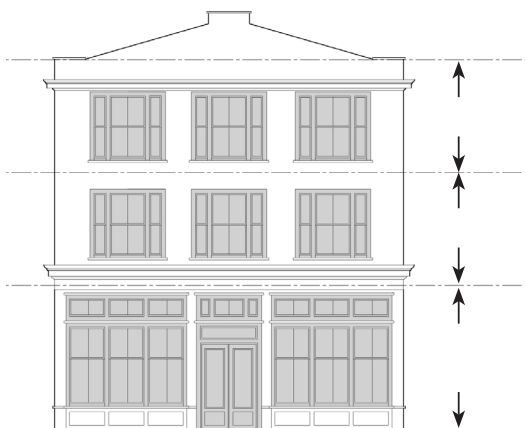
FIGURE 3-3 FAÇADE TRANSPARENCY REQUIREMENTS FOR BUILDINGS WITH SHOPFRONT.
