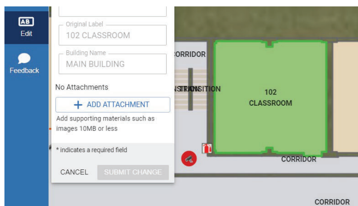
Figure 2 - Rooms and Points of Interest can be relabeled directly by the customers for efficient availability of updates to public safety.
