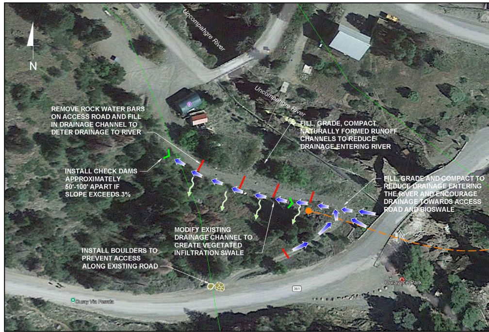
1 PROPOSED EROSION CONTROL PLAN SCALE: 1"=30'
