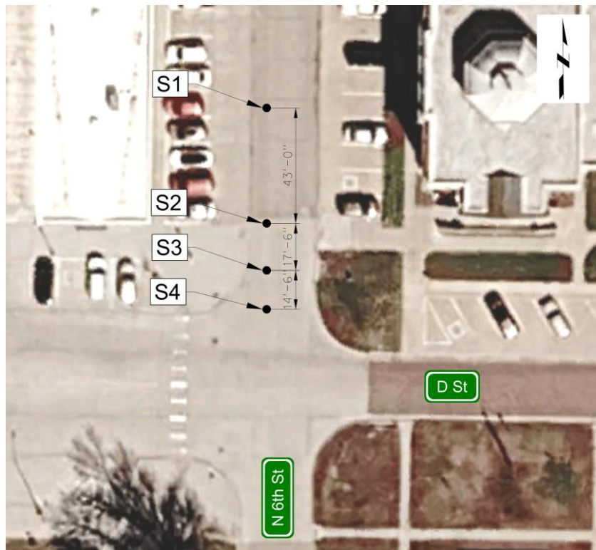
Figure 2: Northbound Sight Distance Measurement Locations
