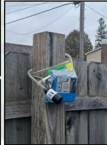
Abatement requires lining trucks, special disposal and air monitoring.
