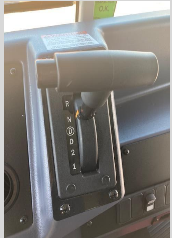
Allison 5-Speed select shift transmission.
