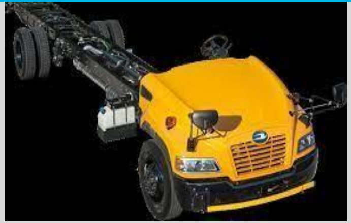
Purpose built Blue Bird OEM chassis.
