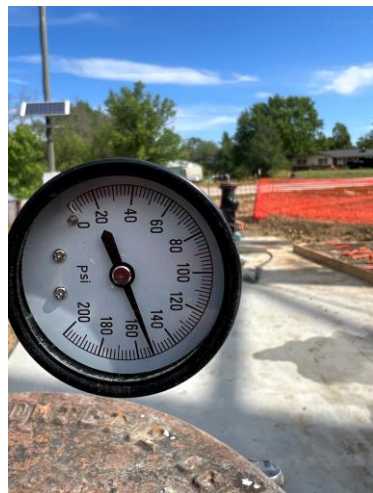
5/8: Pressure at the end of the test - 11:15am.
