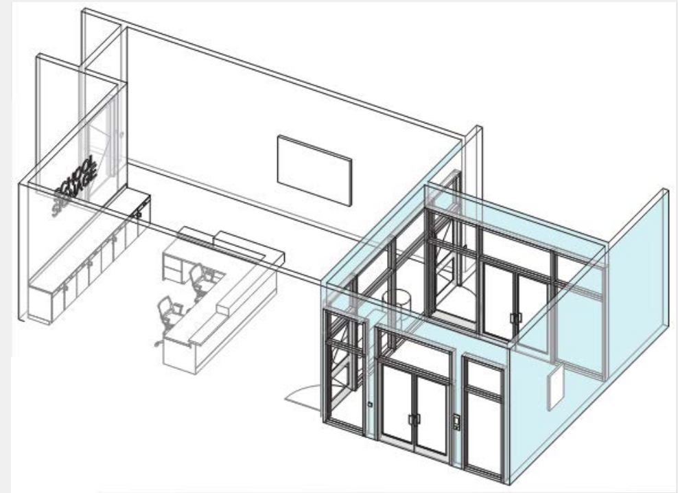
CISD Design Guidelines - Typical Secure Vestibule Upgrade
