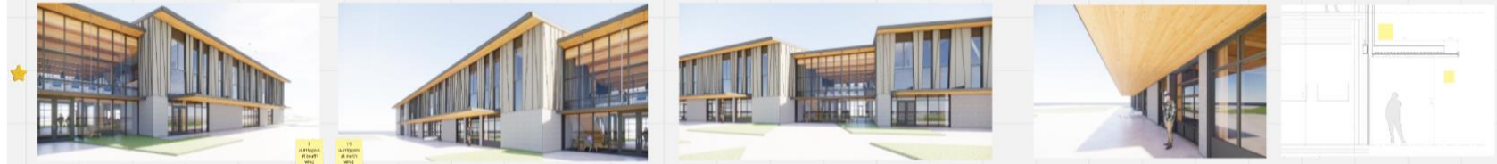
Canopy Study 3: Steel to edge of opening, 6" stud wall, 9' outrigger.
